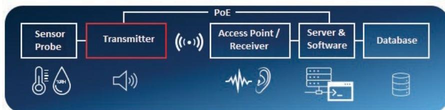
Both TrackView Pro wireless and Power Over Internet (PoE) wired data transmitters are an integral part of any Ellab environmental monitoring system. Each transmitter can accept up to two Ellab SMART probes for measuring parameters such as, but not limited to, temperature, relative humidity (RH), carbon dioxide (CO<sub>2</sub>), differential pressure (DP), door switches, analog sensors with 4-20mA and 0-10V output, digital input and output sensors and more.
